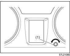
When the engine switch is pressed to change the ignition mode to "ON", the instrument panel lights come on.
